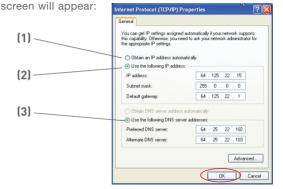
5. If "Use the following IP address" (2) is selected, your Router will need to be set up for a static IP connection type. Write the address information the table below. You will need to enter this information into the Router.
